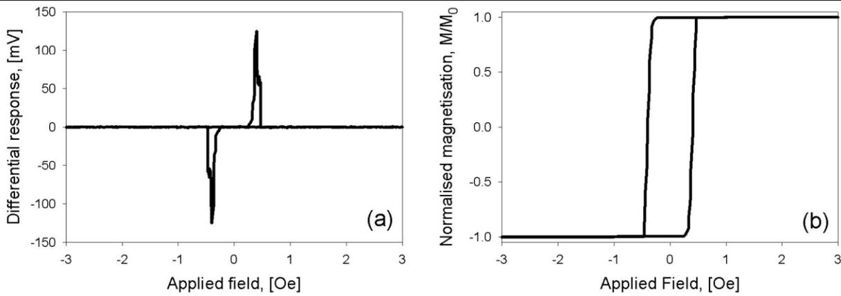
Fig 1 Differential (a) and integral (b) hysteresis loop by large Barkhausen jump.
