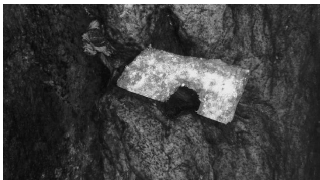
Fig.6. Blue-Green color luminescence of \text{SrAl}_2\text{O}_4:\text{Eu}^{2+} , \text{Dy}^{3+} from 5 meters deep in real sea conditions
