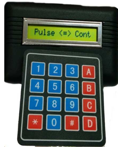
Fig. 3. Control module. Example of user interface.
