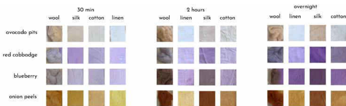
Fig. 1: Bio dye results for simmering the textile in the dye bath 30 min, 2 hours and overnight.
