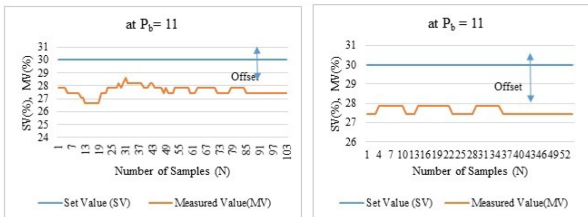
Figure 7. Step response of closed loop control of water flow system for 30 % set value at P_b = 11 .
