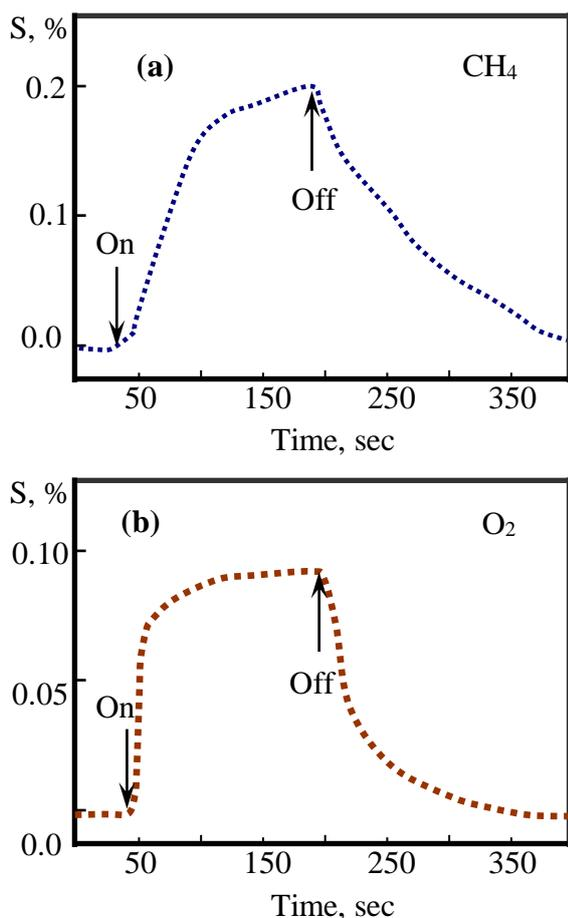
**Figure 4.** Gas sensitivity of single nanorod-based sensor to (a) CH<sub>4</sub> and (b) O<sub>2</sub> gases at room temperature.
