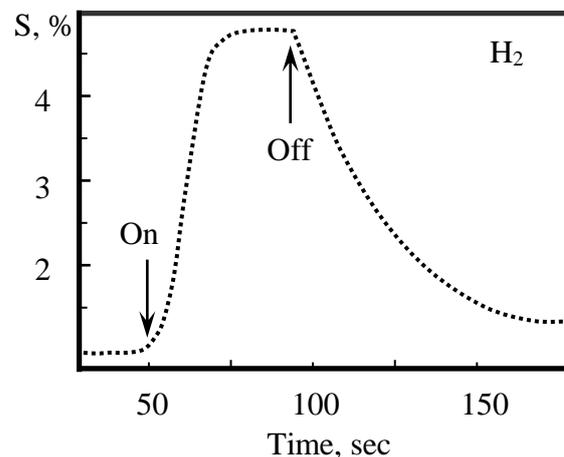
**Figure 3.** Gas sensitivity of single nanorod-based sensor.
