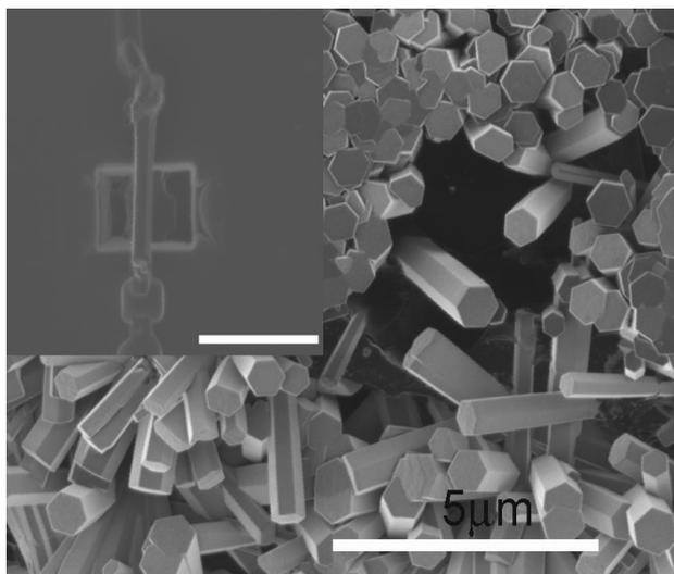
**Figure 2.** SEM images of silver-doped ZnO nanorods. Inset show an individual nanorod-based sensor fabricated by nanolithography in focused ion beam system. Scale bar is 5  $\mu\text{m}$ .
